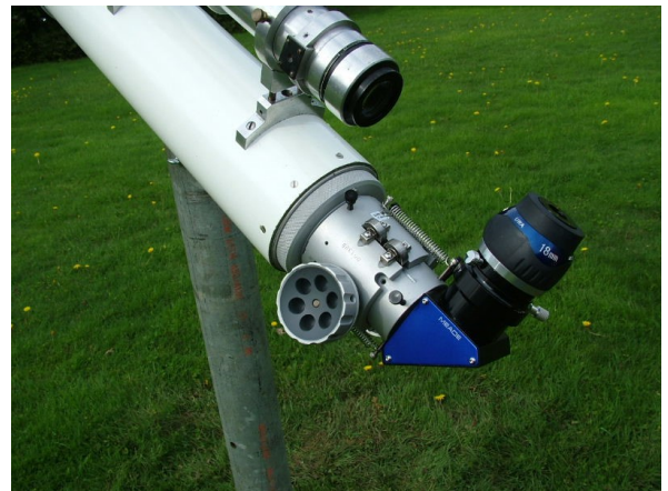
The 2 inch Van Slyke focuser fitted to the Zimmerman telescope. Image by Ron Kalinoski.
