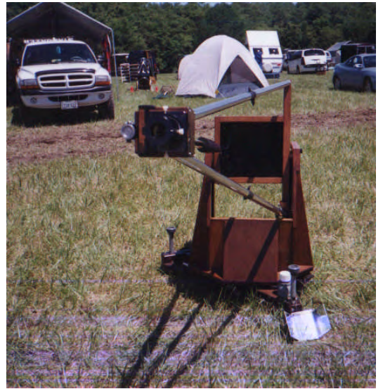
17" f8 unobstructed dobsonian with no secondary mirror.
