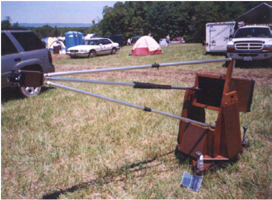
17" f8 unobstructed dobsonian with no secondary mirror.
