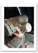
rotted. The 24 inch was used for research and is set up with a Coude focus. There is no eyepiece to observe celestial objects. The light path is directed out of the telescope through the declination axis by a third mirror placed directly in front of the primary mirror, then directed by a fourth and fifth mirror to instrumentation.
