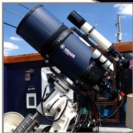
Photos by ACA Member Len Marek 14" Meade LX850 f/8 Televue 102 f/8.6 Televue Genesis sdf f/5.4 SBIG ST8300M camera and Filter wheel Astro-Physics AP1200 mount
